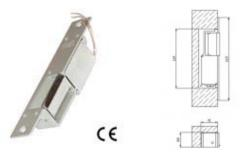
The R2 Electric Strike LEFT is designed for remote opening of left and double-wing doors and gates, in co-operation with the door lock striker. It is made of aluminium alloys and powder-painted. It is designed to be mounted within a doorframe, in which it is possible to make a 28x31x119 mm mounting hole (draw on the right).
